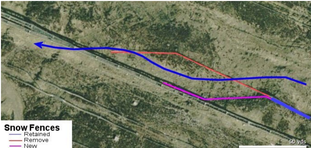
Illustration 3: The contrast in vegetation in this satellite photo shows up the natural snow bed (light colours) and how the existing fence blocks the natural run.
